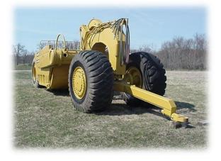
Holmes converted construction grade pull scrapers are made to be pulled with heavy horsepower bull dozers, track tractors, or large wheeled agricultural tractors
